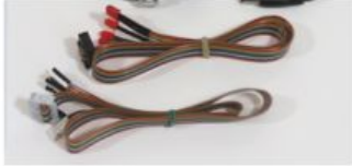
Rainbow cables, one with a grey block connector for touchpoints and the other with a black block connector and 6 red LEDs
